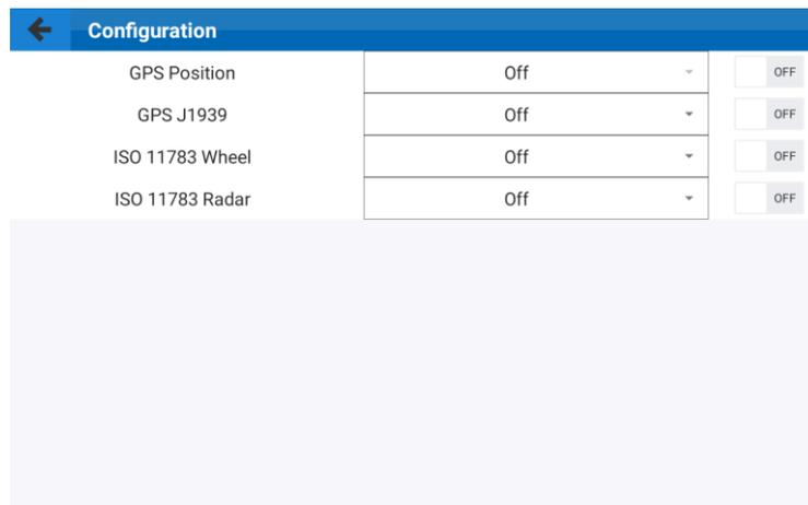
Figure 17. Speed Source Configuration
