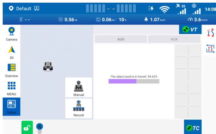
**Figure 9.** Load Object Pool
