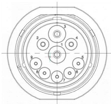
**Figure 5.** Cross-Sectional View of ISOBUS Implement Connector
