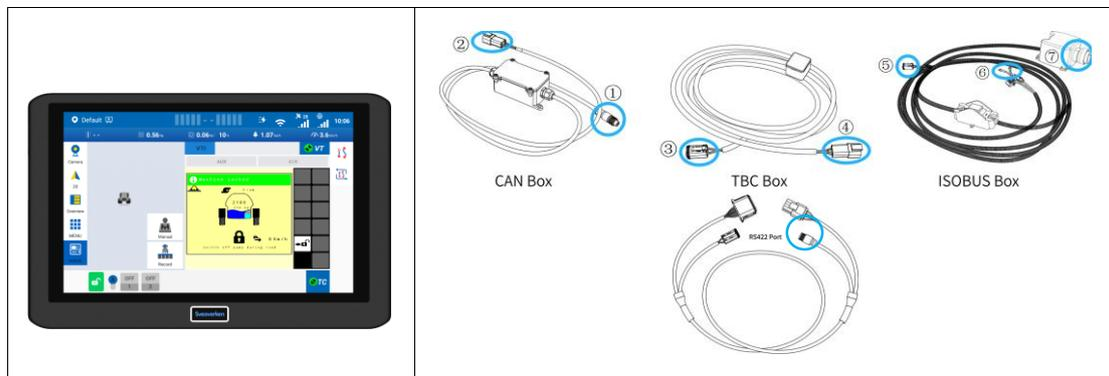
**Figure 4.** Hardware Interfaces of ISOBUS for F100
